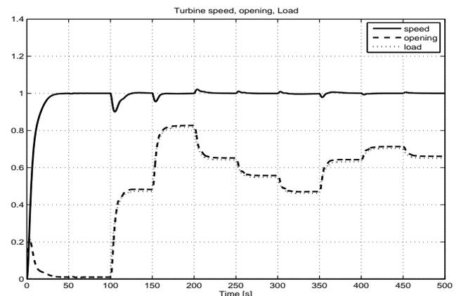
Fig.11 Turbine speed, opening in the case of random load change
