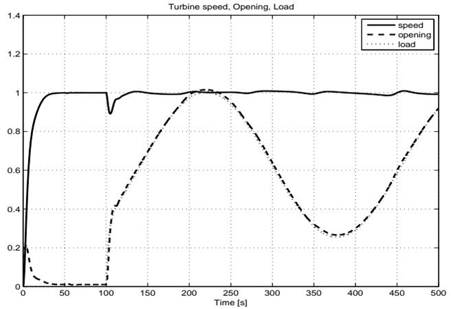
Fig.9 Turbine speed, opening in the case of sinusoidal load change
