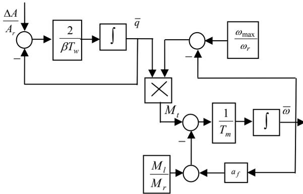
Fig.1 Model of the waterway and rotor dynamics
