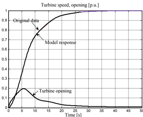
Fig.5 Turbine speed, opening position during initial speeding up (original data and model response)
