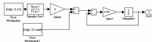
Fig.6 Identification model structure under load conditions
