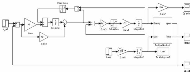
Fig.2 Simulation model of hydro turbine speed control
