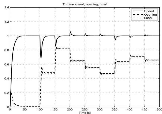
**Fig.13 Conventional turbine control in the case of random load change**
