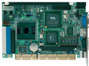
Karta CPU PCISA-C400R s CPU ULV Intel Celeron 400 MHz
