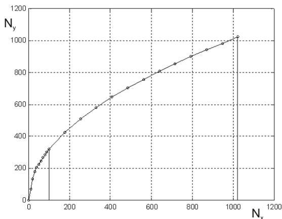
**Fig.8 Inverse characteristics approximation using NIP of degree 1**
