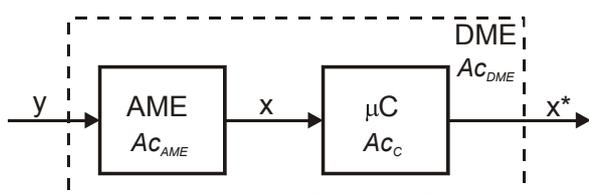
Fig.6 Block scheme of digital measuring element
