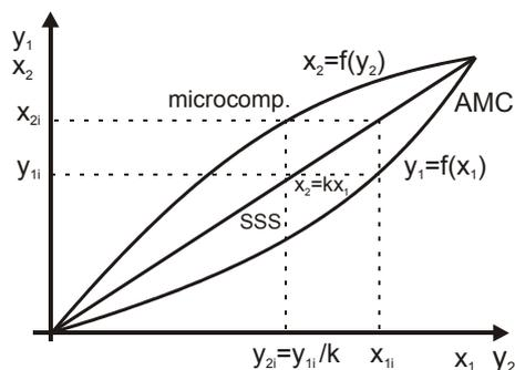
Fig.2 Linearization of sensor characteristic
