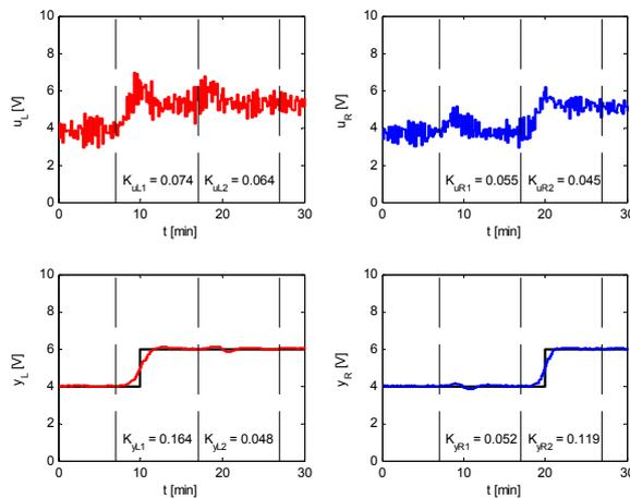
Fig.7 Simulated control with noise – full prediction model,  $T = 1-0,8z^{-1}$
