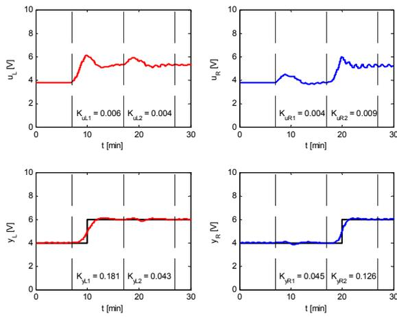
**Fig.10 Simulated control without noise – simplified prediction model,  $T = 1$**
