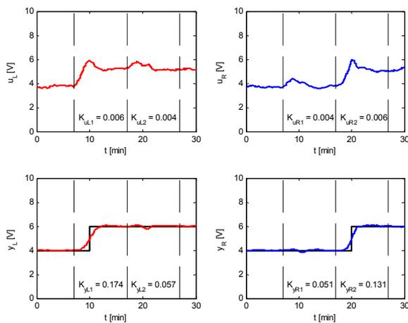
**Fig.12 Simulated control with noise – simplified prediction model,  $T = 1-0.8z^{-1}$**
