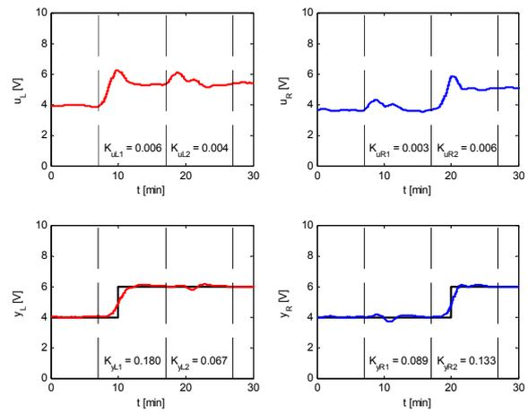
**Fig.13 Simulated control with noise – simplified prediction model,  $T = (1-0.8z^{-1})^2$**
