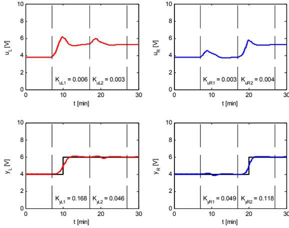
Fig.5 Simulated control without noise – full prediction model,  $T = 1$
