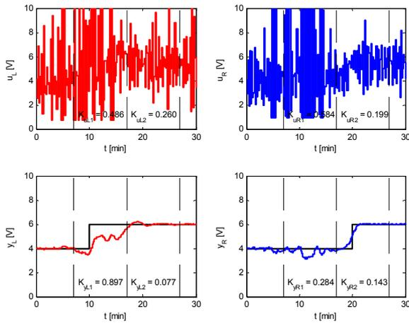
Fig.6 Simulated control with noise – full prediction model,  $T = 1$
