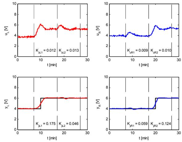
Fig.8 Simulated control with noise – full prediction model,  $T = (1-0,8z^{-1})^2$
