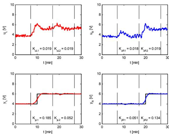
**Fig.11 Simulated control with noise – simplified prediction model,  $T = 1$**
