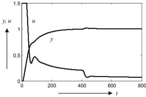
**Fig.5 Control of the plant (2) by the PI<sub>1</sub> controller based on the plant approximation (6)**
