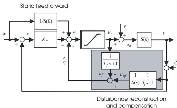
**Fig.3  $PI_1$  controller: P-controller extended by the disturbance reconstruction and compensation**
