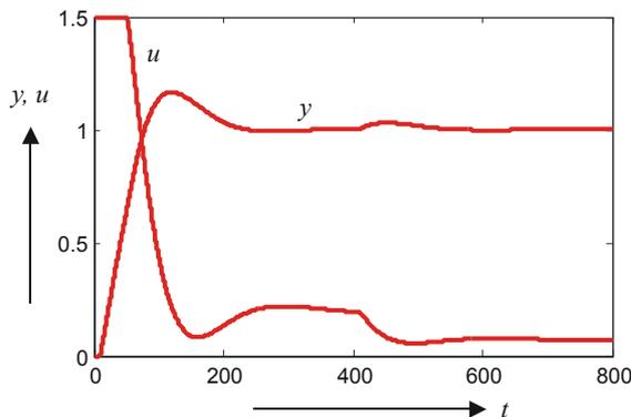
**Fig.6 Control of the plant (2) by the PI<sub>1</sub> controller based on the plant approximation (7)**
