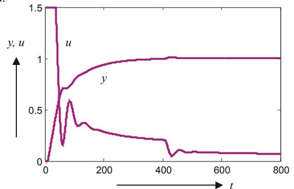
**Fig.4 Control of the plant (2) by the  $PI_1$  controller based on the integral step response approximation (3-4). In the middle of the transient an input step disturbance was applied**
