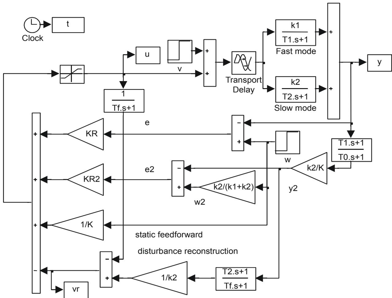
Fig.9 Simulation scheme of the PI<sub>1</sub>-P controller
