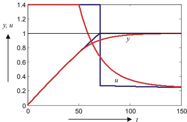
**Fig.7** Transient responses for  $\alpha_1 = -0.05$  (red) and  $\alpha_2 = -20$  (blue)  $k_1=1.0$ ;  $k_2=5.3$ ;  $T_1=184$ ;  $T_2=931$ ;  $T_d=0$
