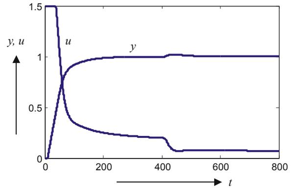
**Fig.8** Control of the plant (2) by the PI<sub>1</sub>-P controller according to Fig.9
