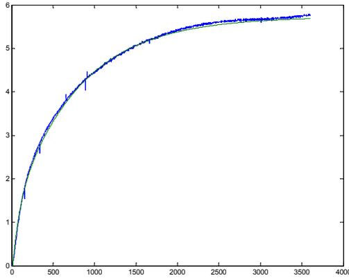
**Fig.2 The measured plant step response and its approximation (2)**
