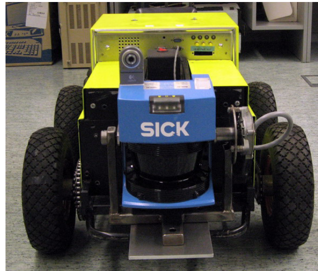
Fig. 1: UTAR robot equipped with the inclining platform
