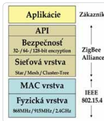
Obr. 8 OSI model ZigBee protokolu IEEE 802.15.4
